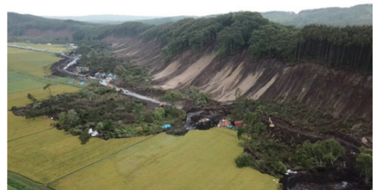
図-12 吉野地区の被災後の斜面と崩土の氾濫の様子 Fig. 12 Eroded slope surface and inundation of mud flow in Yoshino area
