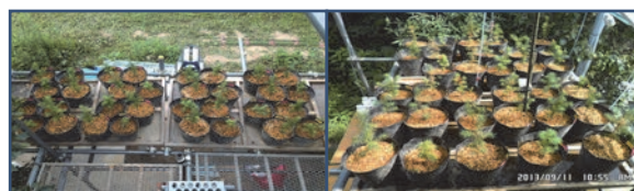
Figure 1 Ambient treatment (left) and Elevated O 3 treatment (right) with a free-air O 3 fumigation system
