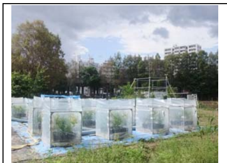
A hand made chambers for fumigation study on birch species (16 chambers)
