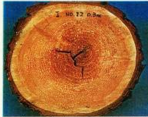
Photo 2. Cross section of a Japanese larch log showing the brown cubical rot caused by Phaeolus schweinitzii at a height of 0.3 m above the ground.
