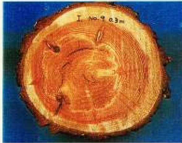
Photo 4. Cross section of a Japanese larch log showing the brown cubical rot caused by Tyromyces balaneus at a height of 0.3 m above the ground.
