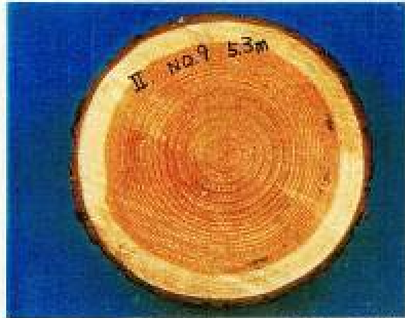
Photo 1. Cross section of a Japanese larch log showing the white stringy rot caused by Stereum sanguinolentum at a height of 5.3 m above the ground.
