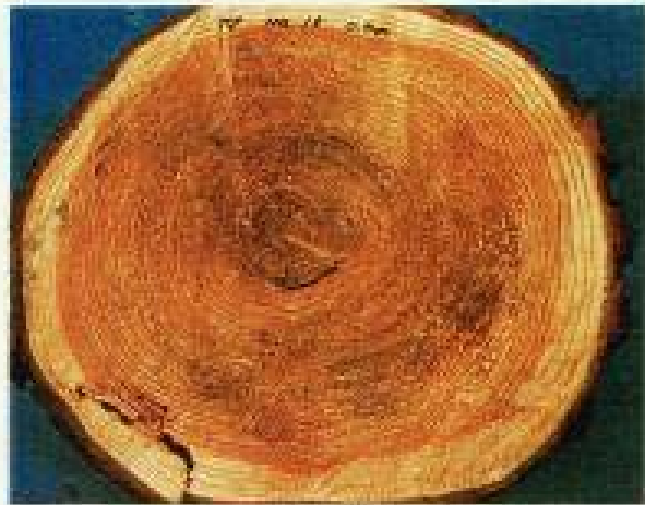
Photo 3. Cross section of a Japanese larch log showing the brown cubical rot caused by Sparassia crispata at a height of 0.3 m above the ground.
