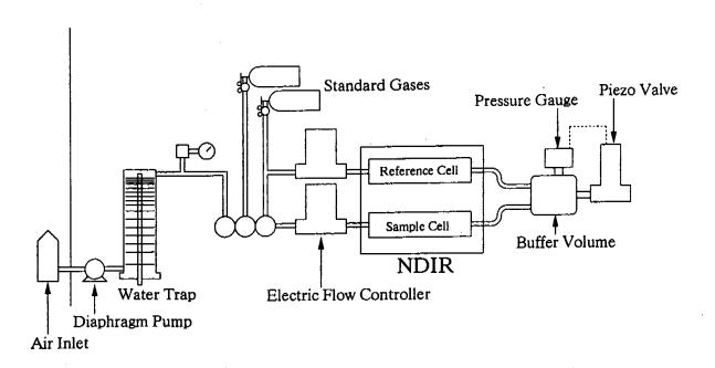
Fig. 1. Schematic diagram of the CO<sub>2</sub> measurement system on the airplane of IL-18.
