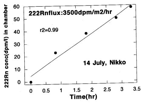
Fig. 1. <sup>222</sup>Rn concentration change with time in the chamber. <sup>222</sup>Rn flux was calculated from the concentration gradient of the regression line.
