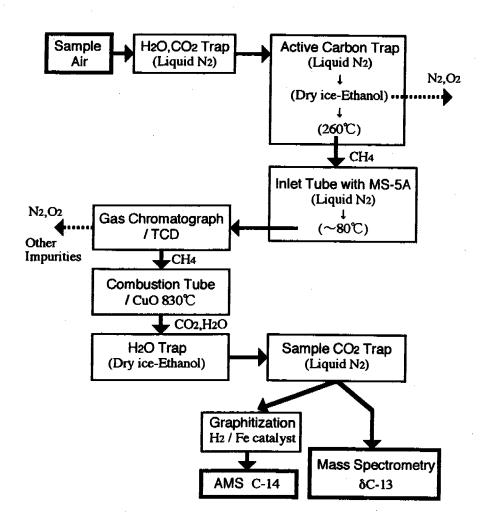
Fig. 3. Schematic diagram of procedure for separation and refinement of methane in the air sample and measurements of its carbon isotopic composition.
