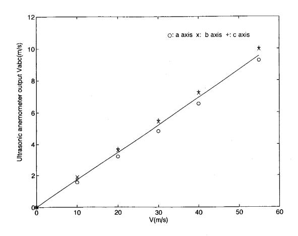
Fig. 5. Comparison between wind tunnel velocity and ultrasonic anemometer output.
