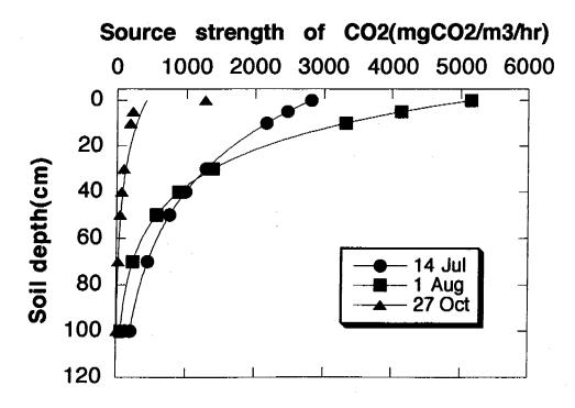
Fig. 4. Source strength of CO<sub>2</sub> in the soil at Nikko site in 1994. Source strength of CO<sub>2</sub> in the soil was calculated from the CO<sub>2</sub> profile and diffusion coefficient by <sup>222</sup>Rn.
