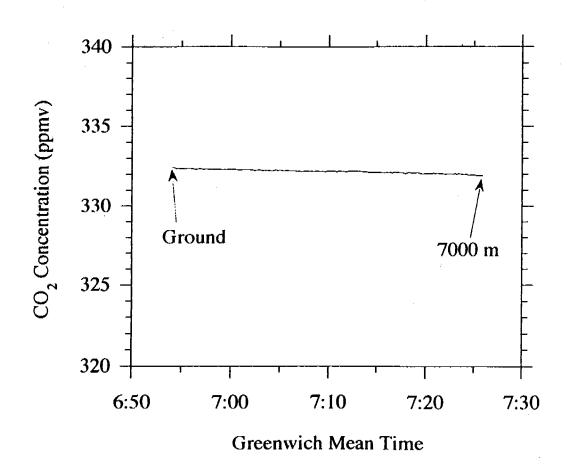
Fig. 2. Variations of the CO<sub>2</sub> concentration in the standard gas measured during ascent of the airplane from the ground level to the altitude of 7000 m.
