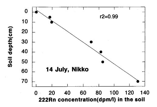
Fig. 2. <sup>222</sup>Rn concentration profiles in the soil. Soil gas was sampled in Nikko site in July 1994. <sup>222</sup>Rn activities were measured by a scintillation counter.
